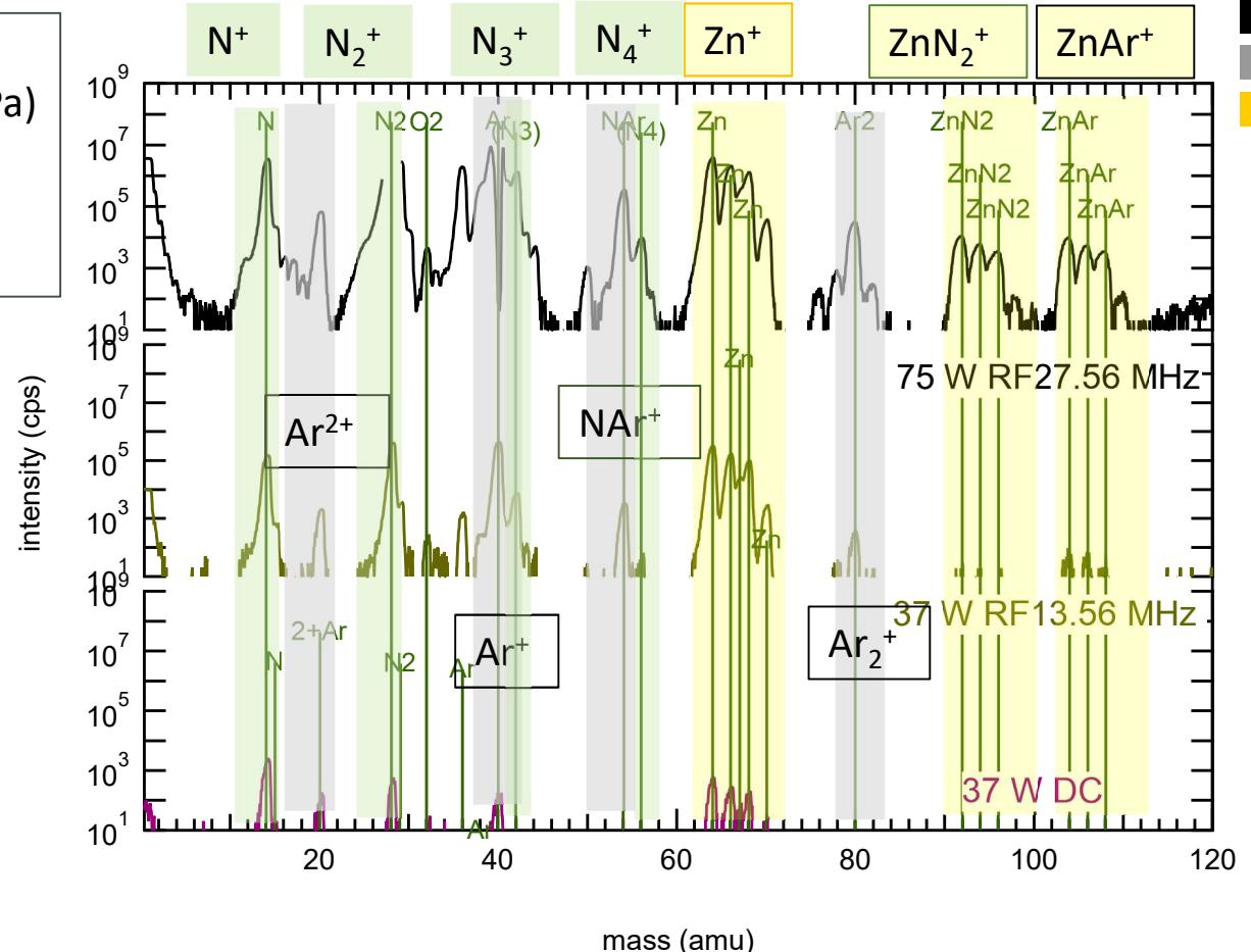
The plasma species were identified using the mass analyzer (EQP) during sputtering in a  $0.5\text{ N}_2/\text{Ar}$  gas ratio. The intensity of atomic nitrogen ( $N^+$ ) and molecular nitrogen species ( $N_2^+$ ,  $N_3^+$ ,  $N_4^+$ , ) increased with rf plasma excitation.
