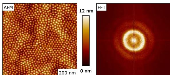
Figure 2: Hexagonal ordered nanodots on Si with a periodicity of 30 nm generated by 500 eV Ar<sup>+</sup> ion beam erosion under 75 deg ion incidence with simultaneous sample rotation. Left: surface topography measured by AFM; right: Fourier transformed height profile.
