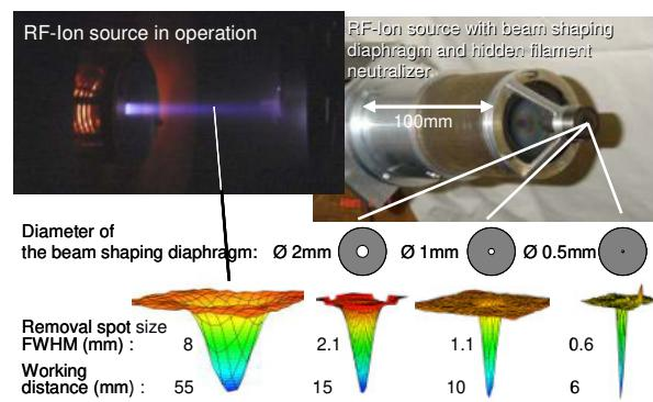
*Figure 5: Measured sizes of the footprints of the beam by interferometry of an etched depletion on fused silica for different operation conditions of the RF ion source without and with beam shaping diaphragms; the etch depths has been normalised in this presentation with respect to the 8 mm spot.*
