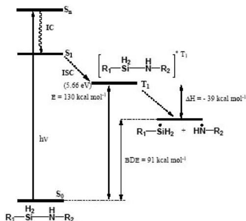
Figure 5: Energy scheme of the hypothetical molecule  $\text{R}1\text{-SiH}_2\text{-NH-R}2$  after photoexcitation.
