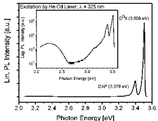
Figure 2: Photoluminescence spectrum of an m-plane oriented IBA-MBE GaN film on LiAlO<sub>2</sub>. Note the strong and narrow (20 meV) near-bandgap transition signal at 3.508 eV.
