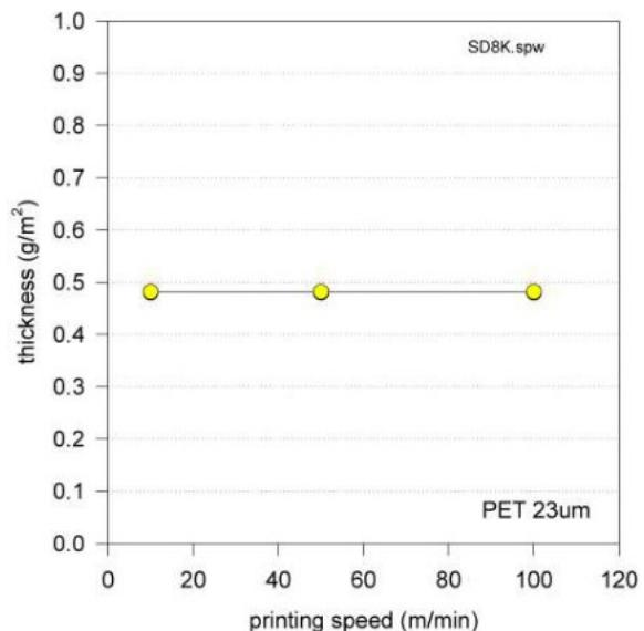
Figure 3: Ink thickness versus printing speed.
