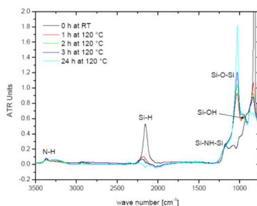
Figure 1: ATR-FTIR spectra of the transformation process of PHPS to silica.
