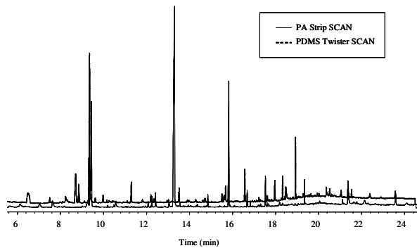
Figure 3: Background scan of a PDMS Twister® vs. a PA strip. In both cases a flat background is obtained spiked with some characteristic deterioration products.
