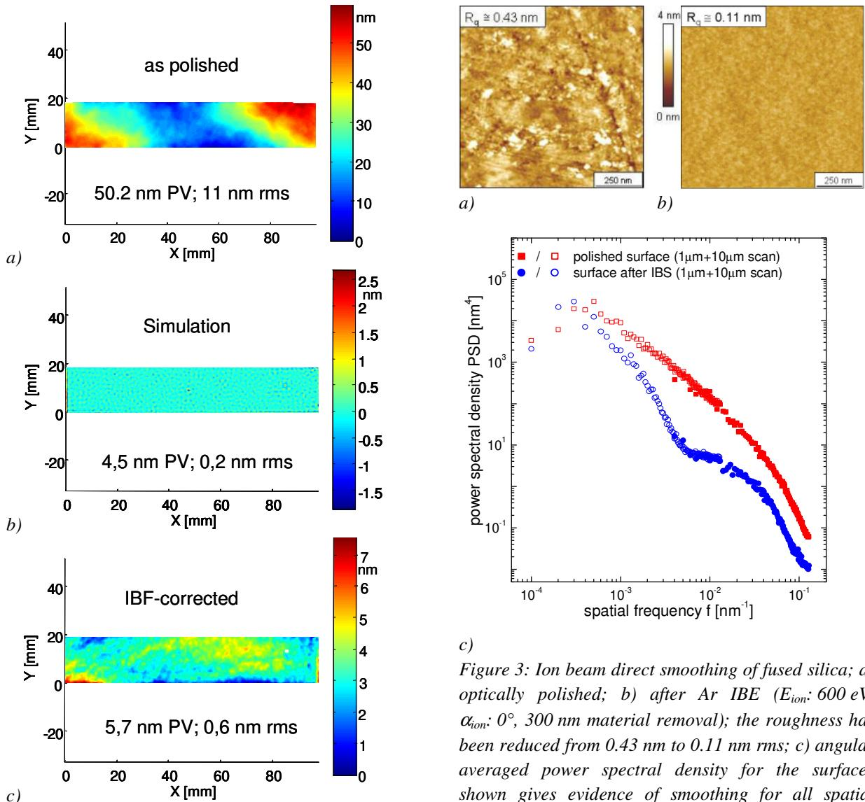
Figure 2: a) Interferometer surface topology measurements of a 100 mm x 20 mm Si plane substrate for a synchrotron beam-line grating as polished, b) computer simulation result for the IBF surface error correction, c) interferometer surface topology measurement of the surface after IBF correction.
