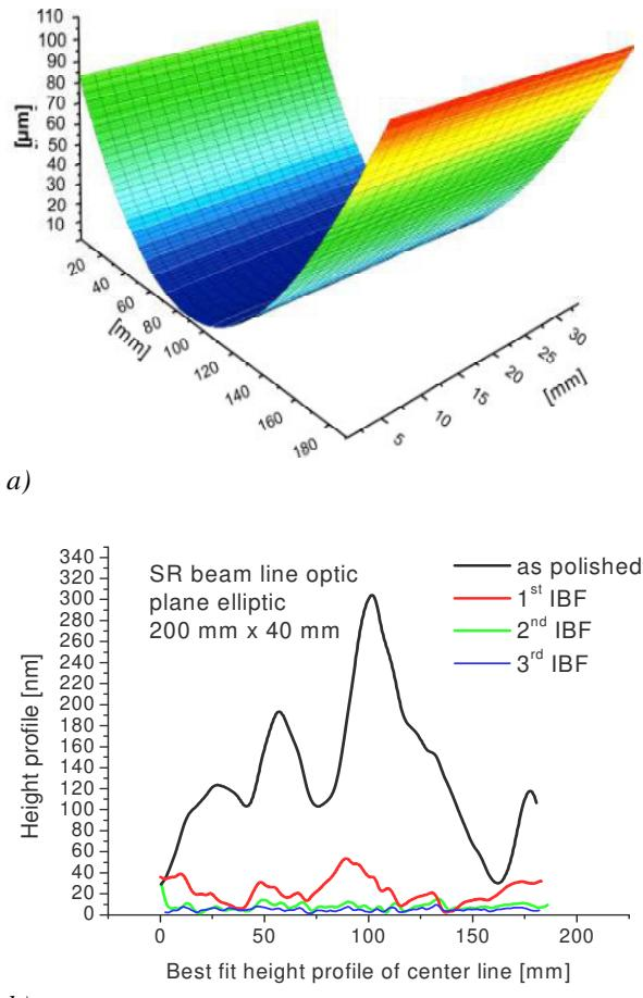
*Figure 1: a) Pseudo 3D presentation of a plane-elliptical surface of a synchrotron-beamline optic stitched from seven adjacent sub-apertures with a 30 % overlap in one direction. Each sub-aperture interferogram was measured with a pixel distance of 0.082 mm, b) best fit height profiles of the plane elliptical mirror.*
