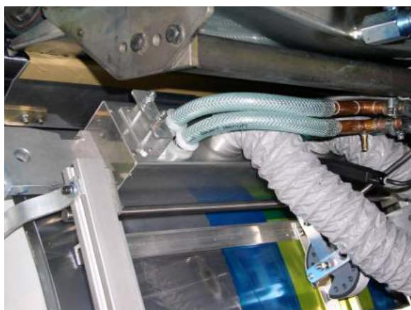
Figure 1: Drying system between the presses.
