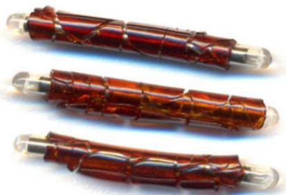
*Figure 2: Thick acrylate coatings crack after heating to 250 °C when applied onto a glass rod due to differing thermal expansion coefficients. The magnet inside the glass rod is left with some expansion space for the same reason.*
