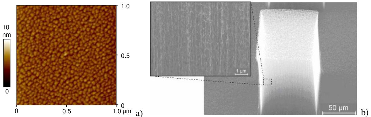
*Figure 3: a) AFM image of a laser-modified surface having a dense film of nanoparticles. b) SEM image of a bundle of vertical grown carbon nanotubes. The local growth of the aligned nanotubes was attained only in the laser irradiated surface areas. Increasing the fluences beyond  $\approx 1 \text{ J/cm}^2$  the particles are removed by ablation.*
