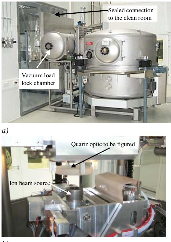
*Figure 4: a) Ion beam figuring plant UPFA1 at the class 100,000 clean room lab in the IOM, b) upper part of the process chamber has been lifted (for easy maintenance work); the five axis system with the ion source and the face down mounted optic on the carrier are shown inside the chamber.*
