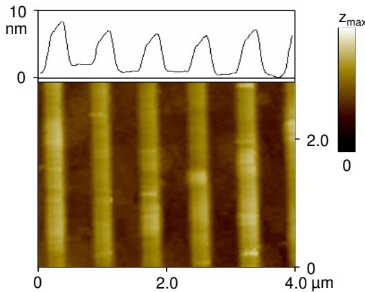
*Figure 2: Sub-micron line gratings on borosilicate glass measured by AFM using tapping mode.*
