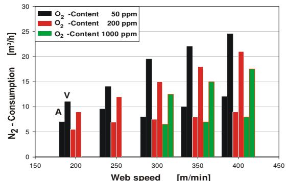
Figure 3: N<sub>2</sub> consumption of “high-speed” inertisation.
