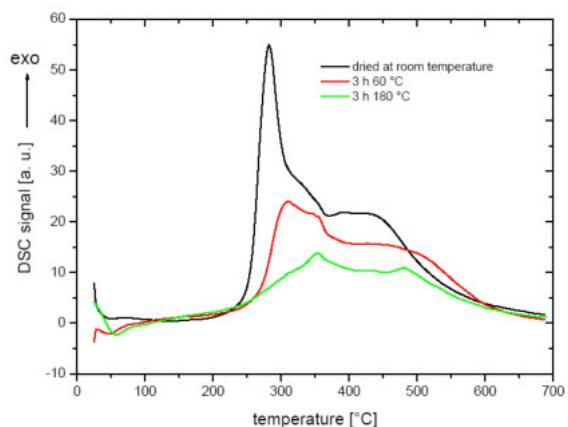
Figure 4: DSC diagram of powder obtained from 3% solution NP110 on glass dried and optionally heated.
