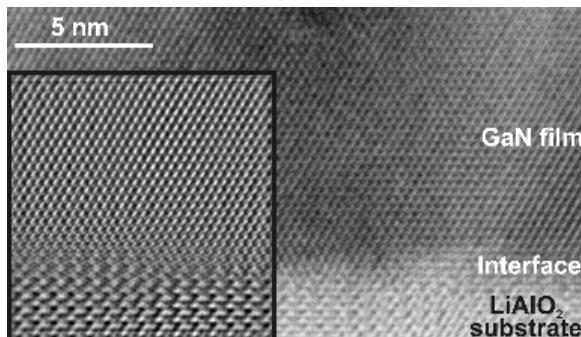
Figure 1: High resolution electron micrograph with zone axis w-GaN[0001] of an m-plane oriented IBA-MBE w-GaN film on LiAlO<sub>2</sub>. The framed region was filtered to emphasise the high crystalline order.
