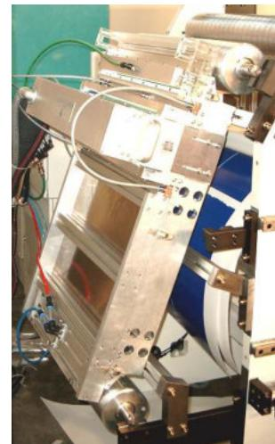
Figure 2: “High-speed” inertisation system with mercury-UV-lamp.
