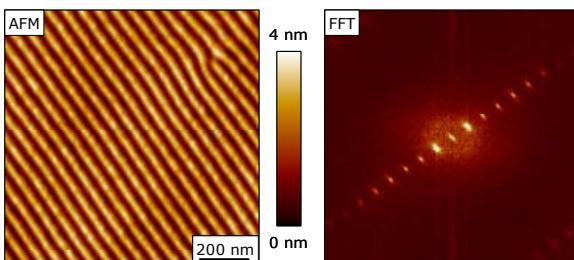
Figure 1: Nano ripples on Si with a periodicity of 50 nm generated by 1200 eV Kr<sup>+</sup> ion beam erosion under 15 deg ion incidence. Left: surface topography measured by AFM; right: Fourier transformed height profile.
