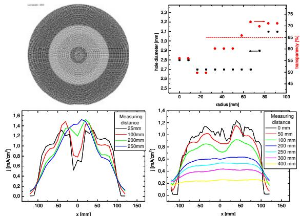
*Figure 4: Modelling (top) on the basis of experimental sheath density distribution measurements (bottom left): grid system with homogenous divergence angle by hole diameter and transparency variation; goal (bottom right): homogenous ion beam density profile at 200 mm distance*
