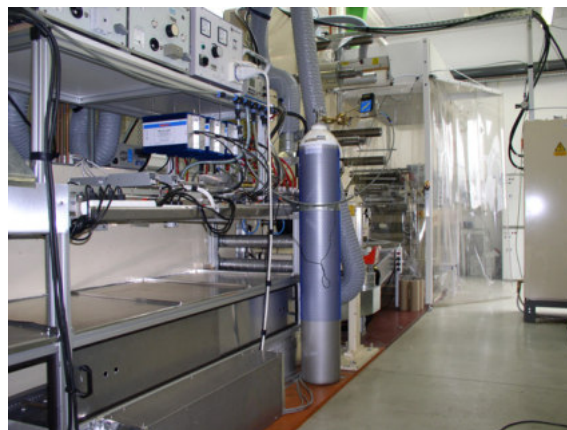
Figure 4: View of a pilot plant for the roll-to-roll production of barrier coatings on 20 cm wide polymer foil at a coating speed up to 10 \text{ m min}^{-1} .
