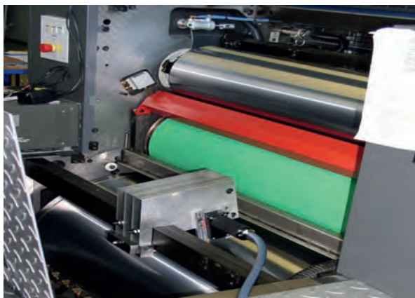
Figure 4: NIR probe head mounted above the impression cylinder of the coating unit of a sheet fed offset printing press.
