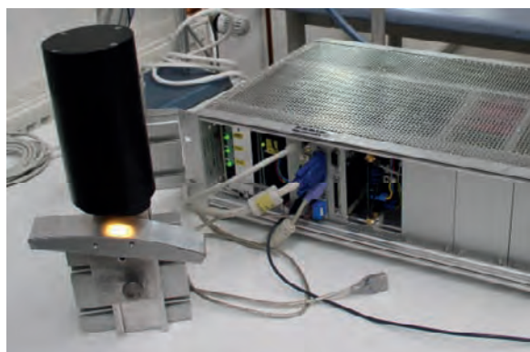
Figure 1: NIR probe head with the metal reflector developed for calibration measurements.
